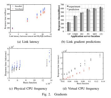
are measured by parsing the front-end web server access logs. Perturbations to link latency are injected by redirecting packetlevel traffic on the application's communication links to the gradient measurement local daemons where it is delayed for a constant amount of time while the perturbation signal is high. Redirection is accomplished through per-node kernel level mechanisms such as the Linux *iptables* packet filter.
