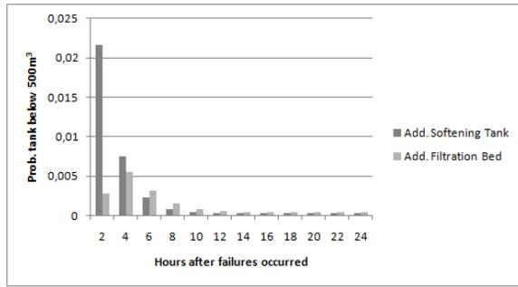
Fig. 5. Probability of service failure (with redundancies)
