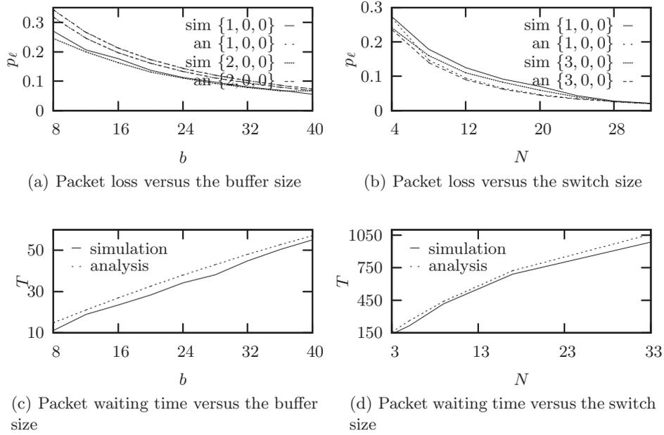
**Fig. 6.** Numerical results for the packet loss analysis of LB switches
