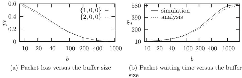
**Fig. 7.** Behavior of switches with large buffers
