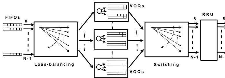
Fig. 1. The load-balancing switch considered for the analysis
