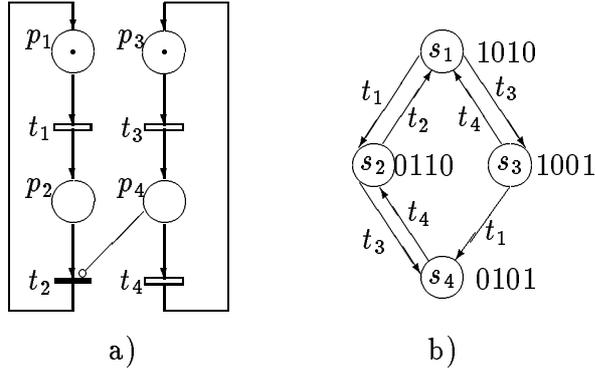
Figure 2: Petri net model of the processor system
