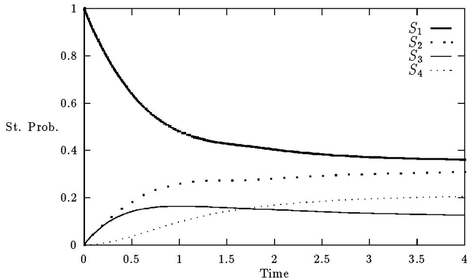
Figure 3: Transient behavior of state probabilities of the processor system
