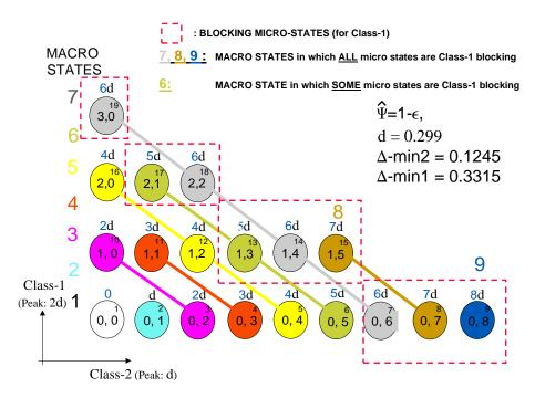
Fig. 1. An example of a state transition diagram with two service classes. There are 19 micro states and 9 macro states. For instance, macro state 6 comprises the Class-1 blocking micro states (2,1), (1,3) and the non-blocking micro state (0,5).
